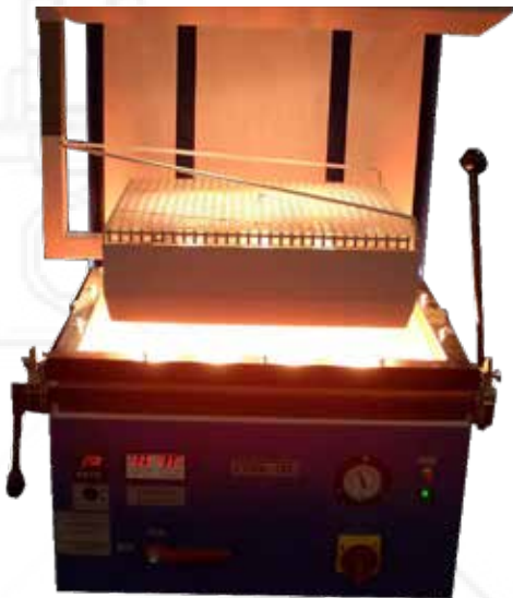
CUSTOMIZED VACUUM-PRESS: VACUPRESS 620S3 with special heating und thermostat control for the photovol- taics filed
