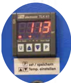
The electronic PID-Controller combined with the optical measuring-unit and the powerful Infrared-heating elements allows exact heating results
